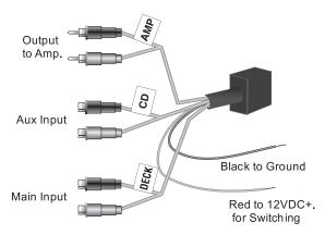
When Red Wire is given 12VDC+, main input (deck) signal is sent to output RCAs (amp). When Red wire is open Aux input (cd) signal is sent to output RCA's (amp). Using a toggle switch to select inputs is recommended.
