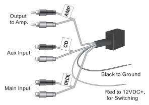
When Red Wire is given 12VDC+, main input (deck) signal is sent to output RCAs (amp). When Red wire is open Aux input (cd) signal is sent to output RCA's (amp). Using a toggle switch to select inputs is recommended.
