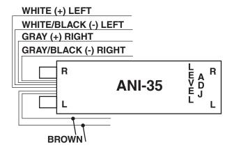
You may connect the ANI-35 either at the factory radio or at the rear speaker wires. You do not need to disconnect the speakers, the ANI-35 will work in conjunction with the speakers.
